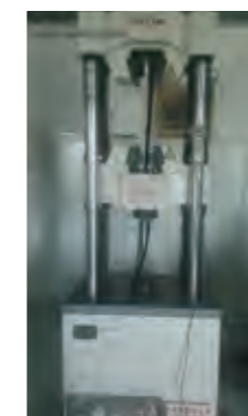
WAW-600型微机控制电液 伺服万能试验机 WAW-600 Servo Hydraulic Universal Testing Machine (Dual space)
