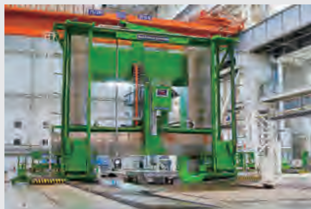
德国科堡8×60米数控双龙门镗铣床 German Waldrich Coburg 8x60 CNC bridge type milling machine
